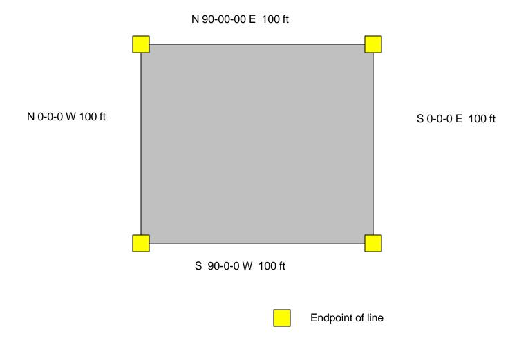
Metes descriptions - perimeter descriptions with a direction of travel described by a series of measurements. Problems include:
